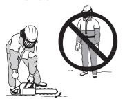
Place the chain saw on the ground and hold the rear handle down with your right foot. Grasp the front handle firmly using your left hand. Make sure the chain saw is steady and the chain is not touching the ground or other objects. Then grasp the starter handle with your right hand and pull the starter cord. **Never wrap the starter cord around your hand**
